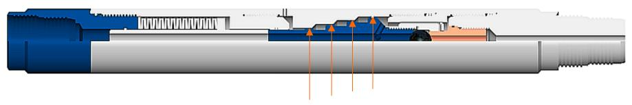
Adjustment to the valve opening setting is achieved by installing a seal on the designated piston groove. The varied piston diameters provide for a selection of cross sectional areas to alter the operating pressure of the valve.
